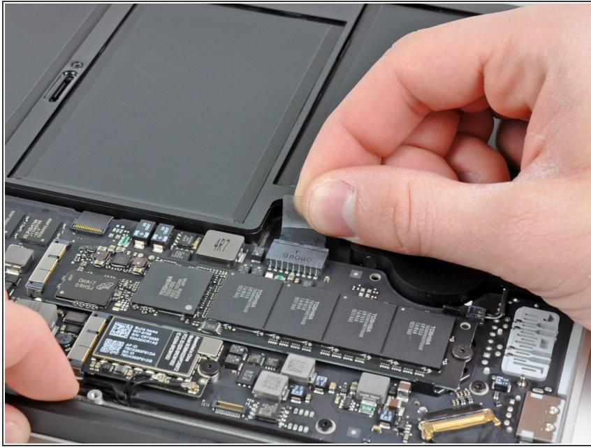
**i** For precautionary purposes, we advise that you disconnect the battery connector from the logic board to avoid any electrical discharge. This step is **optional** and is not required.
